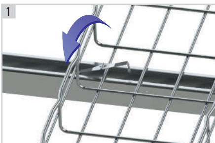
Hook one side of the FS41 into channel support.
