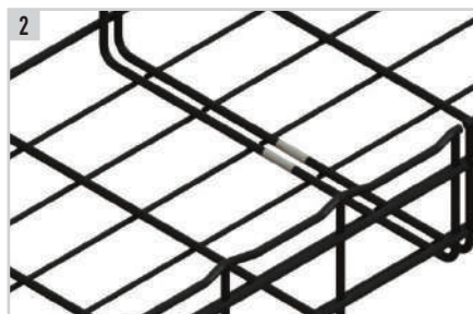
Position tray so that the exposed copper strips are aligned and use SWKs to join tray sections.
