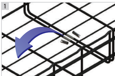
Remove outer mask of copper strip (painted over) exposing the copper strip at each end of the tray.
