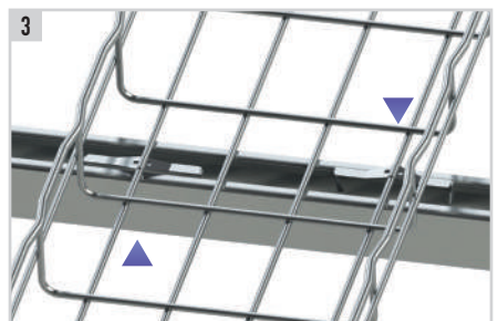
Add an additional FS41 on the opposite side of the channel support for secure installation.
